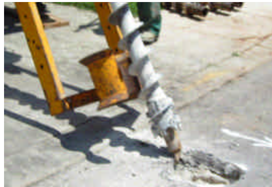
Figure 4. Inclined Magnetometer Profiling to verify PRB thickness
