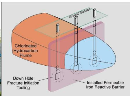
The in situ reactive barriers are constructed from a series of wells installed along the barrier alignment. A controlled vertical fracture is initiated in each well at the required azimuth orientation and depth. Iron filings are injected into the wells in a highly viscous cross linked proprietary HPG gel, to form a continuous permeable iron reactive barrier. The barrier's geometry is monitored in real time by the active resistivity method to ensure the barrier is constructed as designed.
