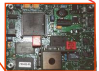
Microprocessor Controlled Switch & Monitoring System
