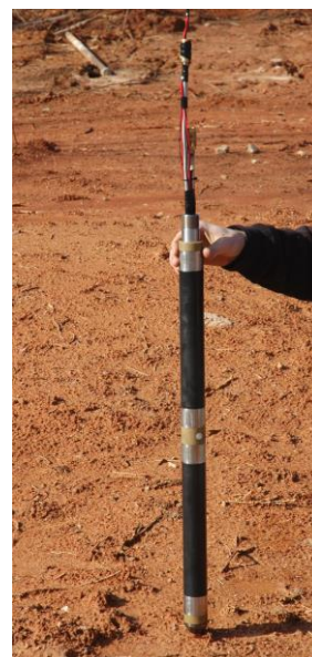
GeoSierra's In Situ Tool for Liquefaction Assessment & Electro-Osmosis Applicability
