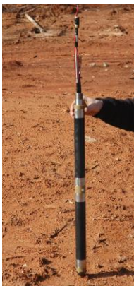
GeoSierra's In Situ Tool Determines Electro-Osmosis Applicability to Site Soils
